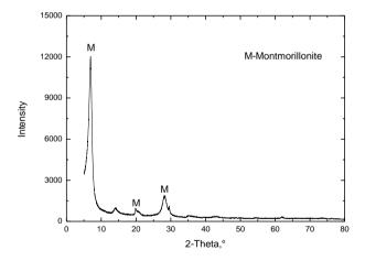
Fig. 1. XRD trace of the colloidal MMT
